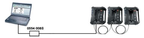
The USB connection via data bus controller is set up directly to the meas. boxes. Before connecting to a bus system, all analyzer units must first be equipped with the identical country version and firmware version.
