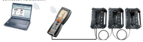
Both the Bluetooth®-modules on PC in the testo 350 must be activated Blue background / white symbol = Bluetooth® on, Bluetooth® connection to meas. box up and running.
