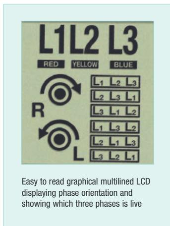
Easy to read graphical multilined LCD displaying phase orientation and showing which three phases is live
