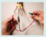
GREEN LED means wiring is properly identified.
