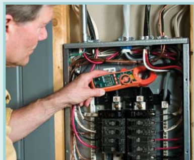
Compact size allows measurements in tight locations
