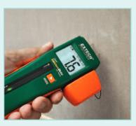
Measures % of Moisture in sheet rock and other building materials using direct pin method. Protective cap snaps onto the side of the housing during use.
