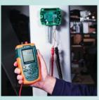
Precision "source" for calibrating process devices.
