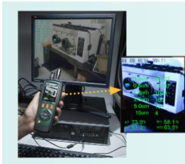
Particle Counter with unique built-in camera for capturing videos and photos that are stored onto internal memory or a microSD™ card. The VPC300 can measure up to 6 channels of particle sizes plus Air Temperature and Relative Humidity. Use the included software to generate reports with videos, photos, and data points.
