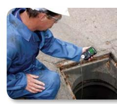
QRAEII Pump being used for a confined space entry
