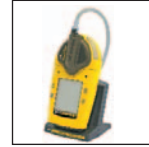
Integral pump and battery charger
