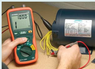
Measures the insulation resistance of motors
