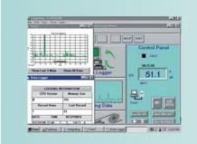
Leq and SEL measurements with built-in datalogger and PC interface. Datalogs up to 32,000 readings using included software and USB cable.
