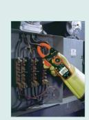
True RMS meter gives you accurate readings of non-sinusoidal
