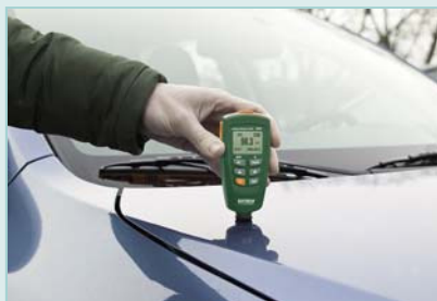
Measuring the thickness of automotive paint
