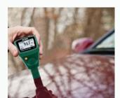
Extech's CG304 offers a non-destructive way of measuring the thickness of ferrous and non-ferrous substrates with auto recognition of the material being measured. Unique Bluetooth<sup>®</sup> interface feature wirelessly transmits measurement data to your PC for further analysis and to generate a documented report.
