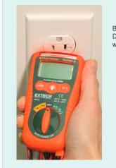
Built-in Non-Contact Voltage Detector. Red LED bar lights when live wire detected.
