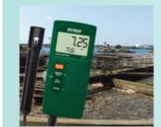
Compact handheld Conductivity Meter with long life carbon rod combination electrode measures Conductivity, TDS and Temperature. Units of measure include  $\mu$ S/cm, mS/ cm, ppm, °F, and °C. The meter features three ranges for Conductivity and TDS plus adjustable Temperature compensation factor to maintain accuracy.
