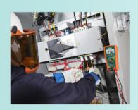
True RMS provides accurate readings when measuring distorted or noisy waveforms. Choose a model designed for Electrical, HVAC, or Industrial Applications. Advanced LoZ feature eliminates false readings caused by ghost voltages. CAT IV safety rating ensures the highest level of protection.
