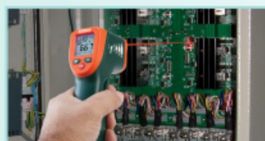
Detect hot spots on circuit breaker panels
