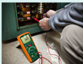
Checking voltage on a lathe
