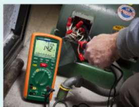
Insulation test on pump motor
