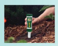
Rugged waterproof (IP57) housing with Flat Surface Electrode for measuring pH in liquids, semi-solids, and solids. Does not break or get junctions clogged like traditional glass bulb electrodes. Easy to replace sensor is perfect for field or lab use.
