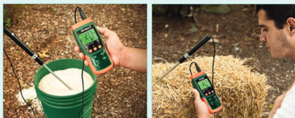
Monitor humidity content in rice, hay, grain, and other materials
