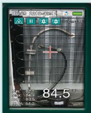
Large 2.2" color video LCD displays measurement area with temperature/humidity, min/max/avg, date, and time stamp
