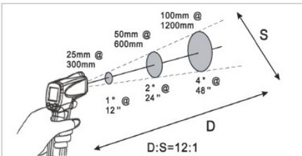
It is necessary to ensure that the size of the target is larger than the spot size. The smaller the target, the closer the distance should be. See the accompanying diagram.
