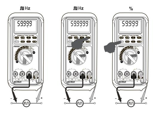
Note: Unlike the Line Level Frequency measuring function as previously stated, this Logic Level Frequency function is set only at the highest input sensitivity for measuring digital type electronic signals.
