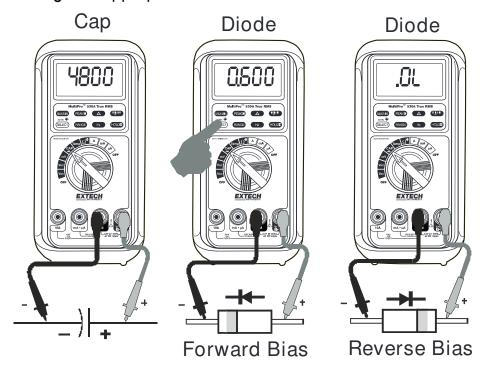
Normal forward voltage drop (forward biased) for a good silicon diode is between 0.400V to 0.900V. A higher reading indicates a leaky diode (defective). A zero reading indicates a shorted diode (defective). An OL indicates an open diode (defective). Reverse the test leads connections (reverse biased) across the diode. The digital display shows OL if the diode is good. Any other readings indicate the diode is resistive or shorted (defective).
