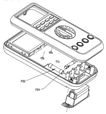
Fuse replacement (and also Battery replacement for splash proof version without battery access door):
