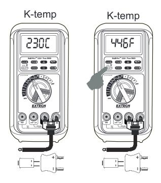
Note: Be sure to insert the banana plug K-type temperature bead probe with correct + - polarities.
