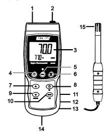
**Notes:** Items 11 – 13 are located behind the snap-off compartment cover on meter's right side. Battery compartment, tilt stand, and tripod mount are located on the rear of the instrument
